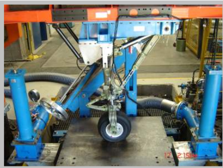
Phenom 300 Nose Landing Gear Drop Test
