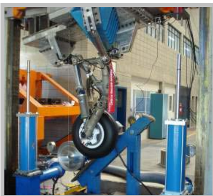
Phenom 300 Main Landing Gear Drop Test
